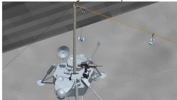
Operational configuration – Mast deployed for payload offloading
